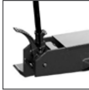
FOOT PEDAL ASSIST FOR EASY LIFTING
